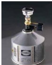
While these burners are relatively easy to use and function much like a Bunsen burner, they are not recommended. They do have separate adjustments for gas and for air; however, the cartridges are not rechargeable and must be replaced once the gas is used up, making them more expensive to use than Bunsen burners and a concern to the environment.
