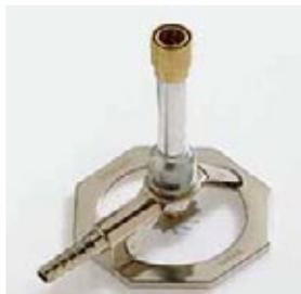
Bunsen burners provide a direct and very efficient source of heat for laboratory purposes: however, there is a risk of burns, particularly to student fingers and hands. If the burner is used to heat water or a solution, the rapid heating can cause hot liquid to bubble out as it reaches its boiling point. In general, Bunsen burners would not be the preferred source of heat in Early Years settings and might also be avoided in Middle Years.
