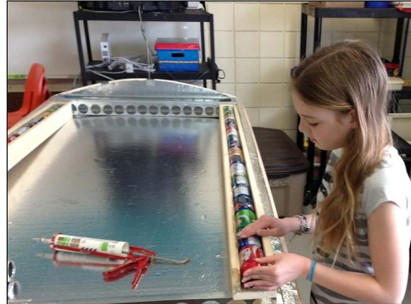
The pop cans were glued together to make convection columns in the pop can solar heater.
