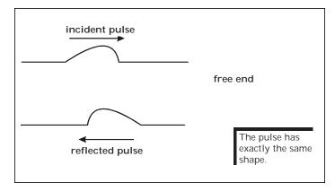
Demonstration of fixed-end reflection is easy. However, demonstration of reflection from a free end is much more difficult because of the damping effect of the wave. Videotape and frame-by-frame advance can be used to reveal same-side reflections.
