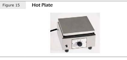
Electric hot plates with thermostatic controls provide a safer, controllable, and reliable source of heat that meets the needs of science courses; however, they can still cause burns to skin. In addition, coiled hot plates, which might still be in use in some schools, have greater potential to cause burns because of the exposed coils. Hot plates require a long time to completely cool before they can be handled safely.
