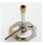
Bunsen burners provide a direct and very efficient source of heat for laboratory purposes: however, there is a risk of burns, particularly to student fingers and hands. If the burner is used to heat water or a solution, the rapid heating can cause hot liquid to bubble out as it reaches its boiling point. In general, Bunsen burners would not be the preferred source of heat in Early Years settings and might also be avoided in Middle Years.
