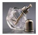
**These burners must not be used in any classroom or science laboratory at any grade level**. There have been countless accidents from this type of burner. Alcohol is both odourless and invisible when burning. Teachers and students have been seriously burned by filling alcohol burners that have hot wicks.
