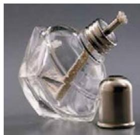
**These burners must not be used in any classroom or science laboratory at any grade level.** There have been countless accidents from this type of burner. Alcohol is both odourless and invisible when burning. Teachers and students have been seriously burned by filling alcohol burners that have hot wicks.
