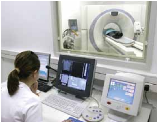
Figure 1-17 Similar to an x-ray machine, a CT scanner has a flat bed for the patient to lie on. The bed slides into the “donut hole,” where one section of the ring contains a source of x-rays that radiate outwards in a fan shape. The other section of the ring contains a banana-shaped detector. This ring can rotate around the patient. One full rotation produces one cross-sectional slice or “profile.”
