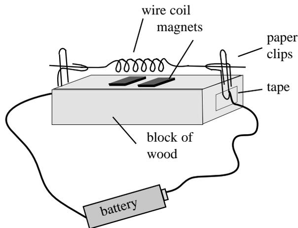
3. Attach a paper clip to opposite sides of the block so that half the clip is sticking up above the block. The top part of the paper clip should be bent downward in the middle so that it will support the wire from the coil.
